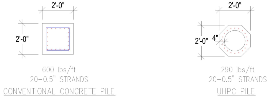
Figure 3- Comparison of conventional concrete pile with UHPC pile of the same flexural capacity. Note, UHPC has higher compressive capacity and better resistance to pile driving effects
