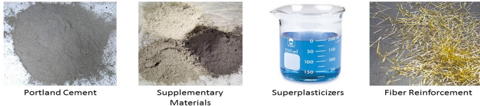
Figure 2- Components of Ultra-High Performance Concrete (UHPC)
